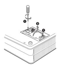
4 Insert the new lamp all the way in until it is securely in place. Tighten the screws. Fold the handle.
