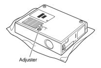
**2** Slide switch **A** in the slit in front of the adjuster in the direction of the arrow (toward the front panel of the projector) with the small minus screwdriver.
